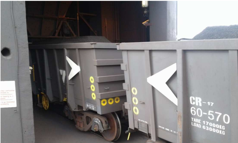
Figure 7.2. Dust-free Loading at UMK
